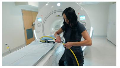
Hose to Lift Connect Connect the two hoses together using the quick connector.
